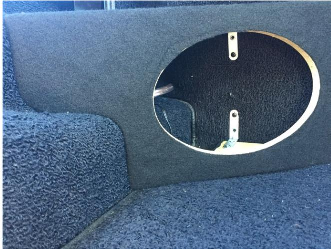
Remove the passenger side dash panel to access radio wiring. Wires should run behind the passenger side kick panel, then under the door sill to the rear compartment area where they will be attached to the speakers.
